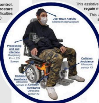
Fig. 1 Collision detection using Raspberry Pi and Ultrasonic sensor
